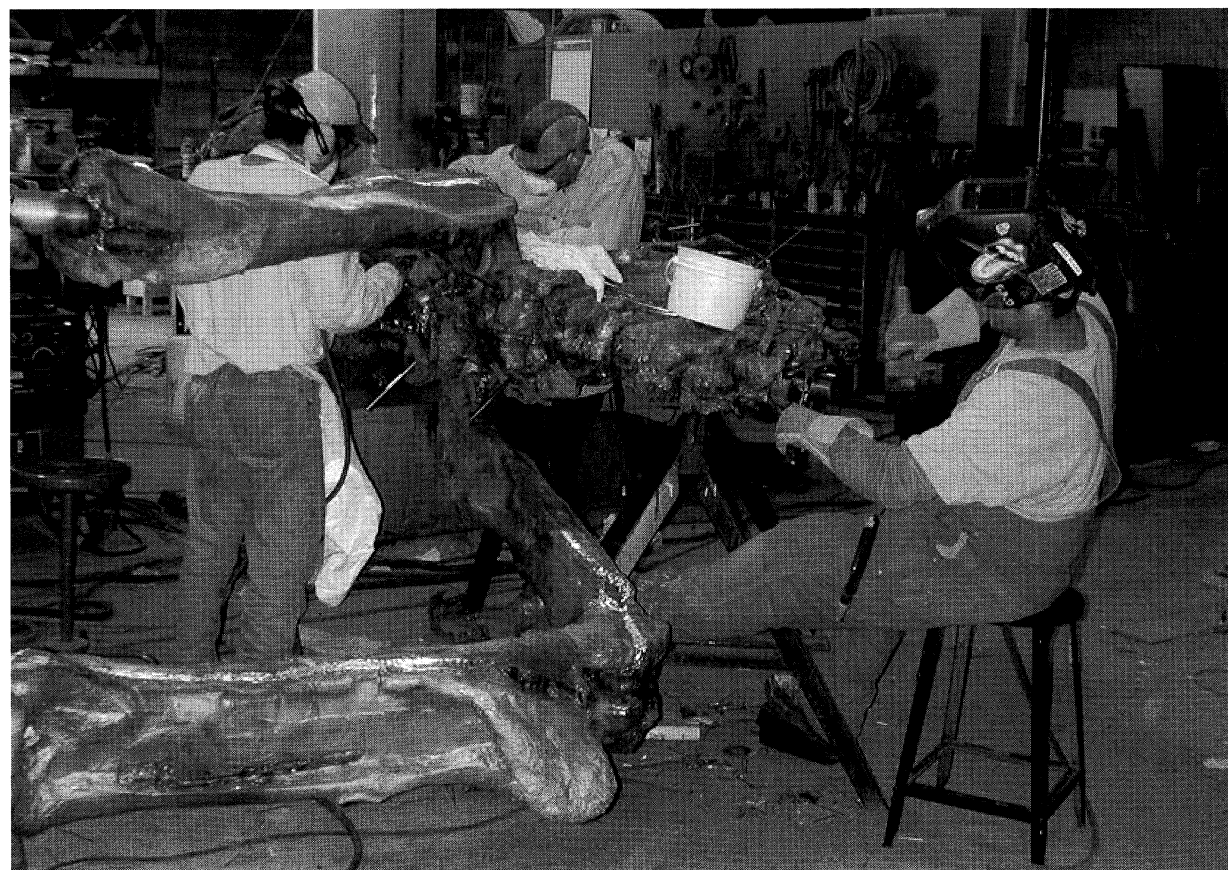
T-rex. fitting, welding and chasing of the hips
